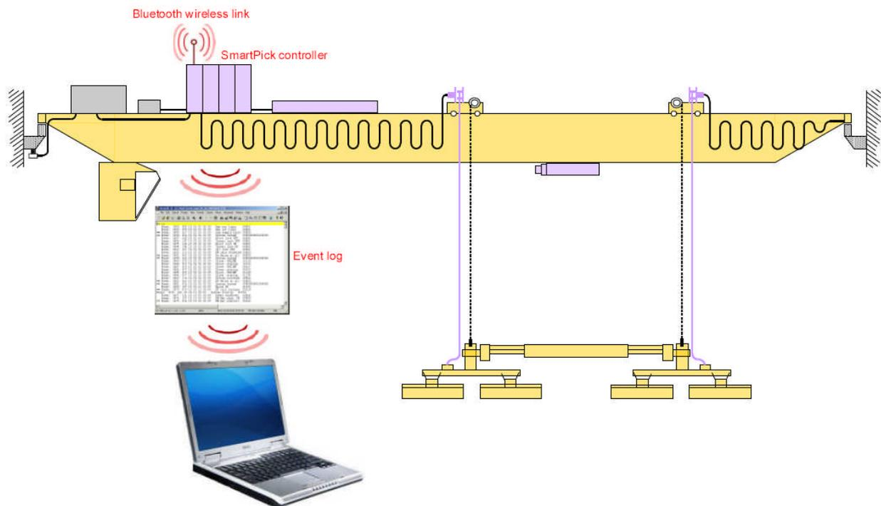
Figure 1: Accessing the event log via a Bluetooth link
