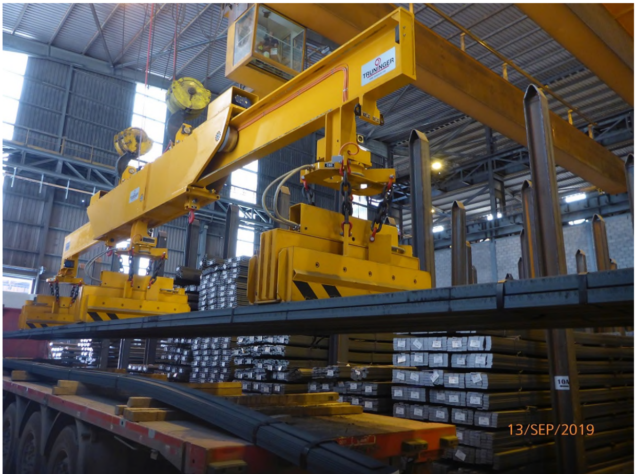
Fig. 3 Redundant magnet system for bar bundles
